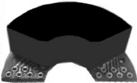
The VFR-1 recorder is a miniaturized, shock hardened, microprocessor controlled, low current, programmable, solid-state data acquisition system. This recorder is hardened for acceleration and vibration, to reliably collect data during applications up to 25,000 G's when properly packaged. Depending on the sensor and interface used, many types of information can be collected, including dynamic and static pressures, acceleration and vibration, stress/strain, temperature, and more.
