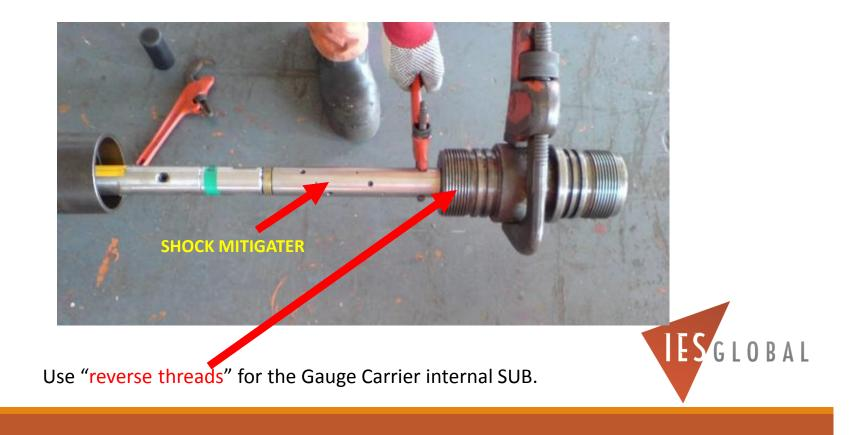
Make sure there are a sufficient number of holes drilled in the Gauge Carrier to allow pressure to reach the Gauge's Pressure Ports unobstructed.
