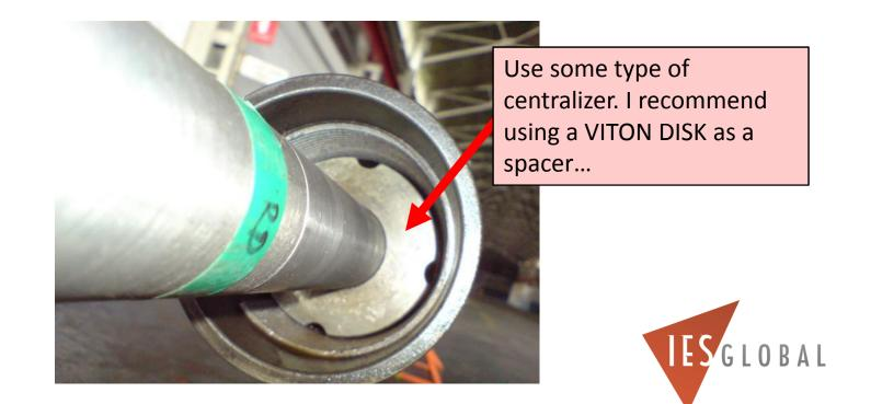
The Gauge body must be "free floating" and MUST NOT come in contact with the inside wall of the Gauge Carrier. Metal on Metal contact between the Gauge and the Carrier could cause excessive vibrations and possibly damage the gauge.
