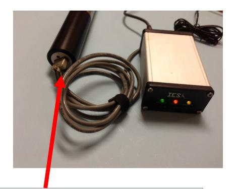
Re-connect the gauge to the interface box and the computer
