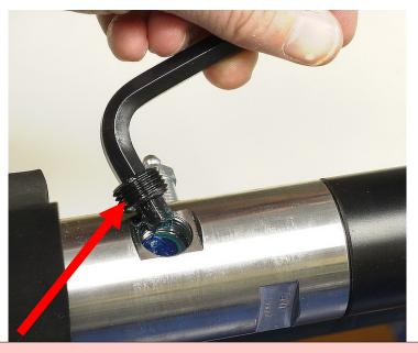
Be sure to re-install both hollow lock nuts!!!
