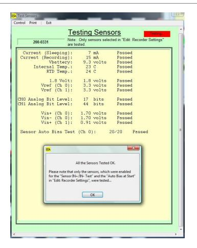
After you select the ENABLE AUTO START option, the gauge will check the batteries and sensors, first. *This will take a few minutes*.
