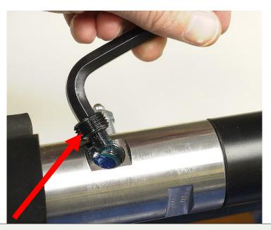
Remove both hollow lock nuts, but leave the washers and micro screens in place
