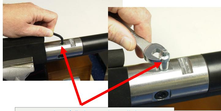
Remove the 1/8" plug, and install the grease gun nipple. Tighten the Nipple with a wrench.
