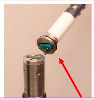
WARNING !!!! If the Battery Fixture is disconnected from the Series 300 gauge <u>BEFORE</u> YOU DOWNLOAD THE DATA, <u>ALL THE DATA will be LOST</u>!!
