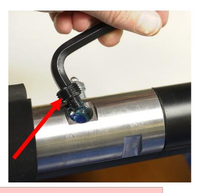
Be sure to re-install bothhollow lock nuts!!!
