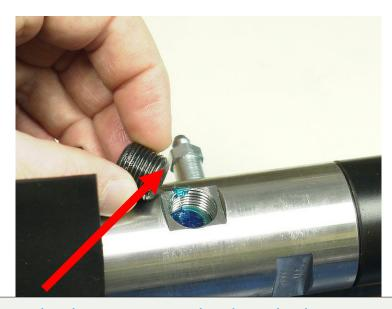
Install the SOLID lock nuts, supplied with the gauge tool box, but leaving the washers and micro screens in place
