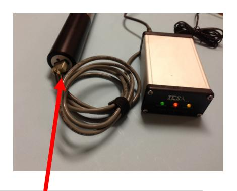
Re-connect the gauge to the interface box and the computer
