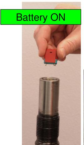
When the "Red Kill Switch" is plugged into the Battery Fixture, it turns OFF the battery power to the gauge!
